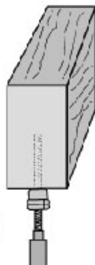
Straight Screws For 3/8" All-thrd rod Min. 1/4" Steel Min 1-1/2" Wood
