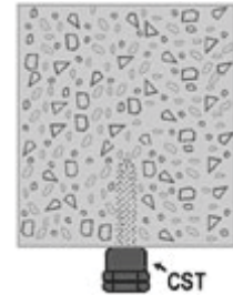
Use 20 ft/lbs torque on nut. For CST use 1/4" bit & drill 2" deep in concrete.
