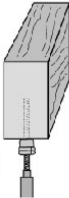
Straight Screws For 3/8" All-thrd rod Min. 1/4" Steel Min 1-1/2" Wood
